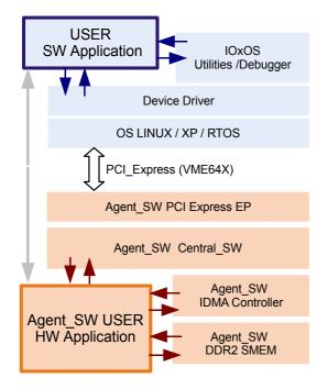
The allocated FPGA user area can be implemented with VHDL or the following high-level tools methodologies in order to fulfill the most demanding applications such as signal processing or high performance computing. Soft IP microprocessors, such as Xilinx MicroBlaze, can be easily integrated in the FPGA user area with full remote control over the PCI Express infrastructure.
