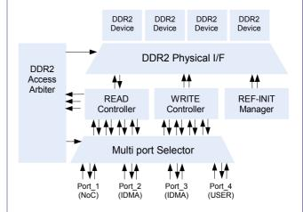
The DDR2 memory array is accessible through the Port\_1 (NoC) for every Agent\_SW connected to the TOSCA Central\_SW .
