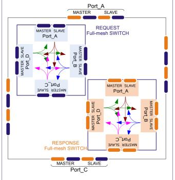
The TOSCA Central\_SW is fully configurable and can be customized from 2 up to 8 ports. A 64-bit 4-port TOSCA Central\_SW (default configuration) running at 200 MHz provides an aggregate bandwidth of 2 x 4 x 1.6 GBytes/s =  $\sim$  12.8 Gbytes/s. Configurations of 128-bit running at 250 MHz are ready to be supported.
