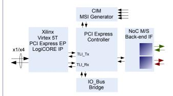
The PCI Express Controller module interfaces the PCI Express EP LogiCORE IP Transaction Layer Interface (TLI) protocol and the onchip TOSCA infrastructure. The TLP packets decoded in I/O Space are sent to an IO\_Bus Master controller, providing a direct mapped access to all Agent\_SW I/O Space area. The TLP packets decoded in Memory Space are reformatted to TOSCA NoC format and sent across the NoC infrastructure. Address remapping and NoC routing are supported through a programmable INgress MMU.
