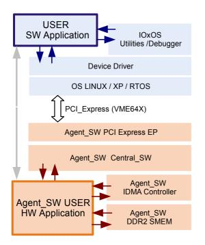
The allocated FPGA user area can be implemented with VHDL or the following high-level tools methodologies in order to fulfill the most demanding applications such as signal processing or high performance computing. Soft IP microprocessors, such as Xilinx MicroBlaze, can be easily integrated in the FPGA user area with full remote control over the PCI Express infrastructure.
