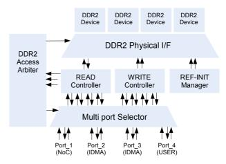
The DDR3 memory array is accessible through the Port\_1 (NoC) for every Agent\_SW connected to the TOSCA
