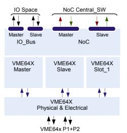
The VME64x Slave module allows to map internal resources over the VME A32 addressing space. A programmable INgress MMU, divided in pages of 1 MBytes, allows to remap the VME addressing space to the internal TOSCA address mapping.
