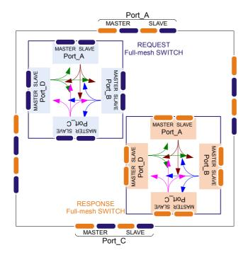
The TOSCA II Central\_SW is fully configurable and can be customized up to 8 ports. A 64-bit 4-port TOSCA Central\_SW (default configuration) running at 250 MHz provides an aggregate bandwidth of 2 x 4 x 2.0 GBytes/s =  $\sim$  16.0 Gbytes/s.
