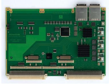
speed path among User Area, PCI Express bus, VME64x bus and Shared Memory. Two on board mezzanine PMC/XMC 42.3 sites with direct path to the User Area, allows local IO or RT computing extension, enhancing the PEV 1100 flexibility to handle a large range of applications
