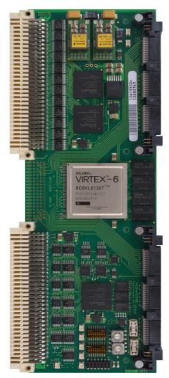
Compared to other products based on mezzanine cards extension (i.e, FMC or XMC), the MPC\_1200 edge-to-edge interconnection solution provides full PCB area utilization, direct VME64x front panel access without any restriction on front panel connectors type, and enhanced air cooling capability with standard heat-sink, while keeping modularity and versatility.
