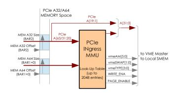
The IO space defined by BAR3 and BAR4 is used to map specific CSR registers, whereas the two Memory spaces defined by BAR1+0 and BAR2 provide direct mapping either to the VME64x address space or to the local Shared Memory (SMEM). A MMU like scatter-gather with local translation table is integrated directly in the PCI Express Slave Interface.
