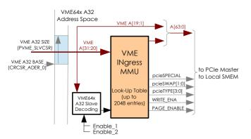
The controller supports the complete set of VME data transaction types (SLT, BLT, MBLT, 2eVME and 2eSST). It also implements a hardware-based byte swapping capability.
